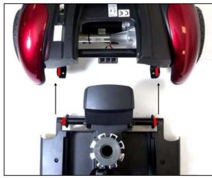
Figure 21. Drivetrain Alignment
