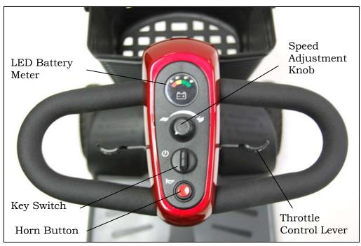
Figure 5. Buzzaround Luxury<sup>™</sup> Delta Tiller Control Panel
