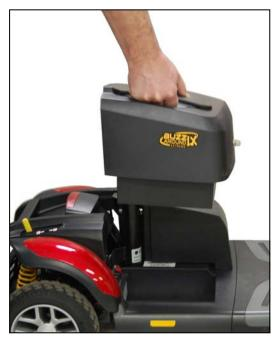
Figure 23. Battery Pack Installation
