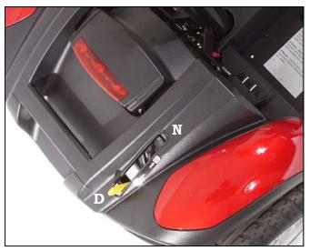
Figure 13: Freewheel Lever (Drive Position)
