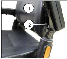
Figure 9. Armrest Angle Adjustment
