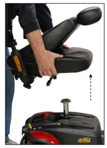
Figure 16. Removing the Seat
