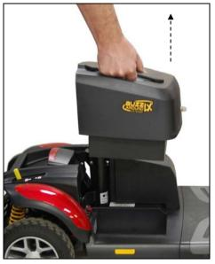
Figure 17. Removing the Battery Pack
