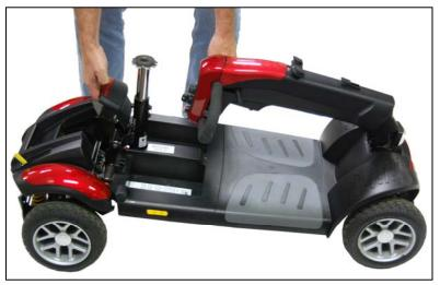
Figure 22. Connecting Frame and Drivetrain
